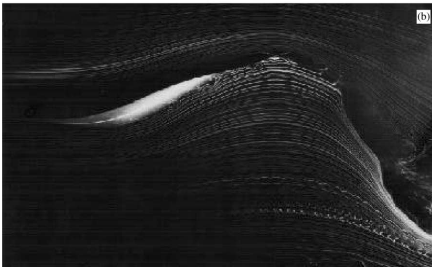
Figure 13. Air-flow around sheet by smoke-wire method: (a) thin paper ( \mu = 0.028 ); (b) thick paper ( \mu = 0.37 ).
